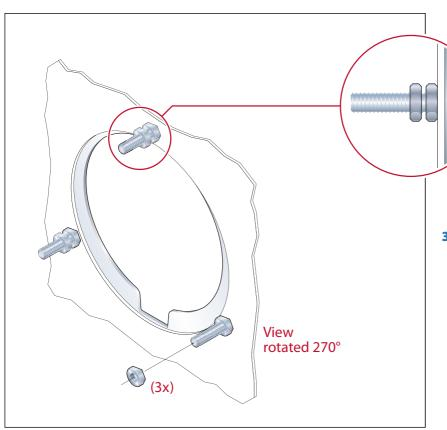
Detail, showing the two (2) 10-32 Nuts mounted on the 10-32 x 7/8" Socket Pan Head Screw.
