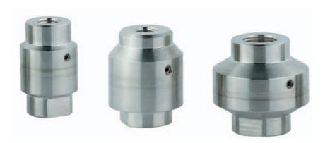
Diaphragm seals are designed to isolate the sensing element of pressure gauges and pressure switches from process fluids that may be corrosive, viscous, sedimentous and/or with a high temperature. The diaphragm is welded to the body, to ensure separation of the filling fluid from the process medium. The threaded connection make it easy to use on all applications where the reduced size of the system is important and also where gauges of 2.5" (63 mm) diameter are required.
