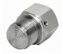
Diaphragm seals are designed to isolate the sensing element of pressure gauges DS 63 and electronic transmitter from process fluids which may be corrosive, viscous, sedimentous and/or with a high temperature. The diaphragm is welded to the top housing and leak proof tested, to guarantee a separation between process fluid and fill transmission fluid. This construction feature and its compact design suits many application that require frequent maintenance.
