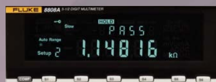
The limit compare mode with pass/fail indicators can help you eliminate production mistakes.
