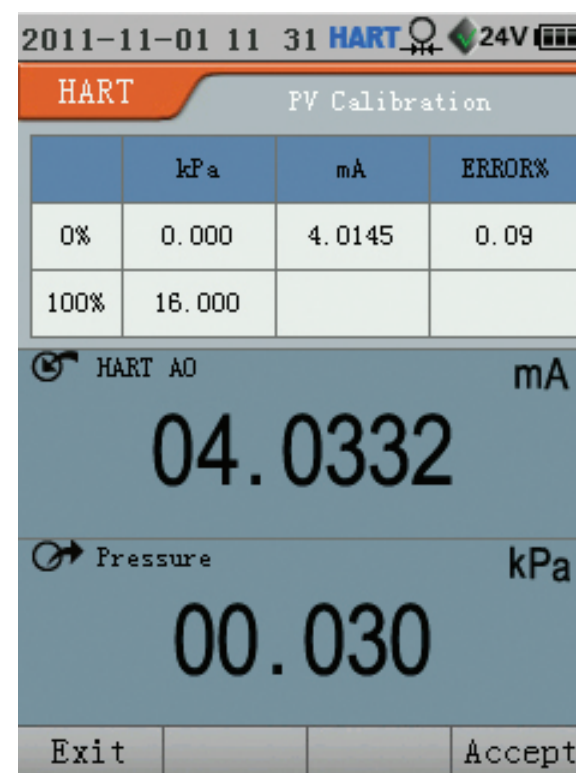
Figure 11.10 HART PV Calibration Process
